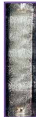
液深が槽径の5倍のフローパターン Flow pattern with liquid having depth five times greater than the tank diameter
