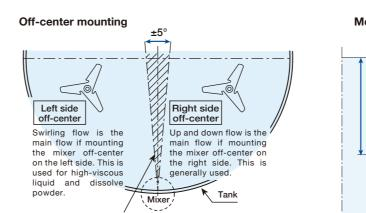
Mounting the mixer within  $\pm 5^{\circ}$  from the center tank is prohibited. Good mixing can be obtained if baffles are installed inside the tank. Please refer Page 23 for the baffle information.
