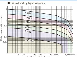
Liquid viscosity (mPa  $\cdot$  s)  $\longrightarrow$ \* Please consult us if the liquid viscosity is more than 1000 mPa·s or the specific gravity is more than 1.2.
