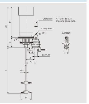
A730 Variable speed type Impeller speed 50/60Hz : 0~420min
