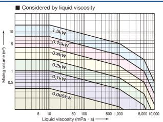
\* Please consult us if the liquid viscosity is more than 1000 mPa s or the specific gravity is more than 1.2. \* Mixing time for uniform mixing in a single phase of liquid-liquid takes more than 5 minutes
