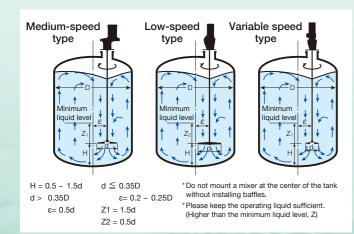
The swirling flow is controlled by the baffles, and up-and-down flow becomes dominant. Since the flow becomes turbulent, the mixing effect is enhanced. Normally, two to four baffles are installed equally near the inner wall of the tank and perpendicular to the rotating flow is most suitable.
