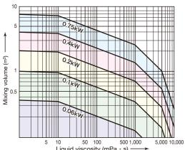
Liquid viscosity (mPa · s) -\* Please consult us if the liquid viscosity is more than 1000 mPa·s or the specific gravity is more than 1.2.
