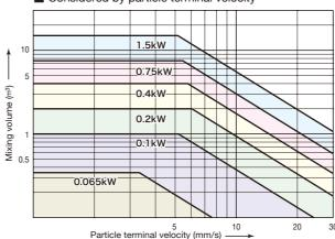
\* Please use this graph as reference. \* This graph shows for the case of liquid viscosity approximately 50 mPa s and specific gravity is 2~3. Please consult us if the ratio of impeller diameter to tank diameter is extremely small (less than 25% of tank diameter)
